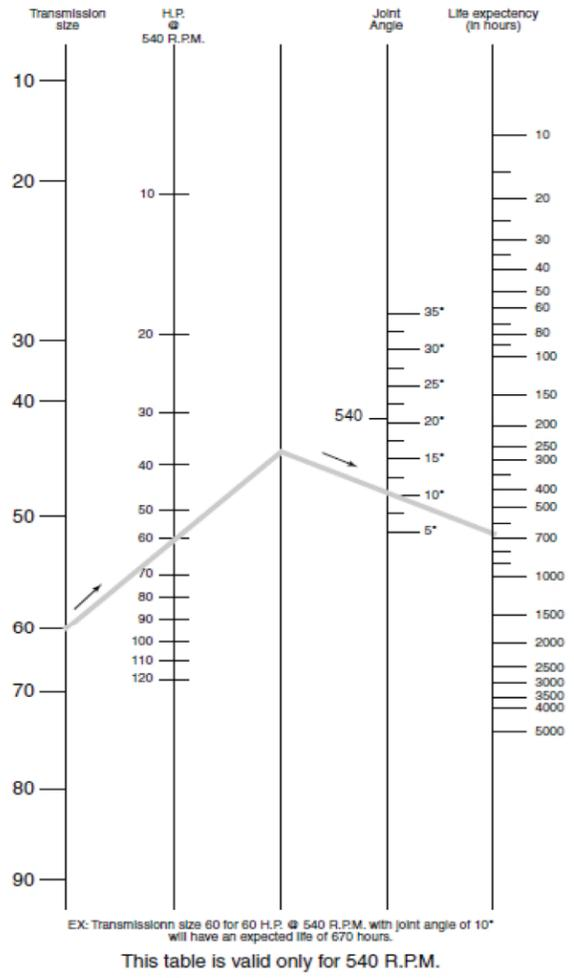
Previous examples clearly demonstrate that universal joint angle is directly related with life of P.T.O. In order to reduce angle, it is necessary to increase the distance between snowblower and tractor
